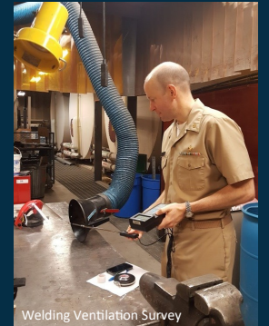
Welding Ventilation Survey
