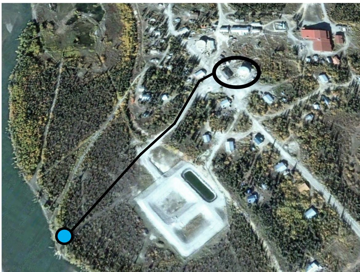
Figure 1: An aerial view of the Venetie water treatment system. The blue circle (lower left) represents the pump house and well. The black line is approximate location of the raw water transmission line and drain port. The water treatment plant and water storage tank are circled in black (upper center). Photo courtesy of Google Earth.
