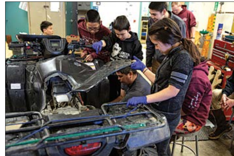
During Chief Ivan Blunka School's Discovery Week, students learned how to maintain and change the oil on all-terrain vehicles, also called Hondas in the community.
