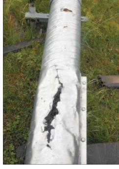
A vehicle damaged Arctic pipe.
