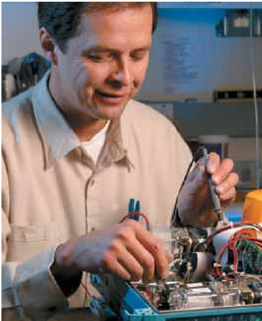
The Consortium provides clinical engineering services for $44 million worth of equipment at 70 sites around Alaska. Above: Medical Equipment Supervisor Burt Hanna repairs an infusion pump used to administer intravenous fluids.
