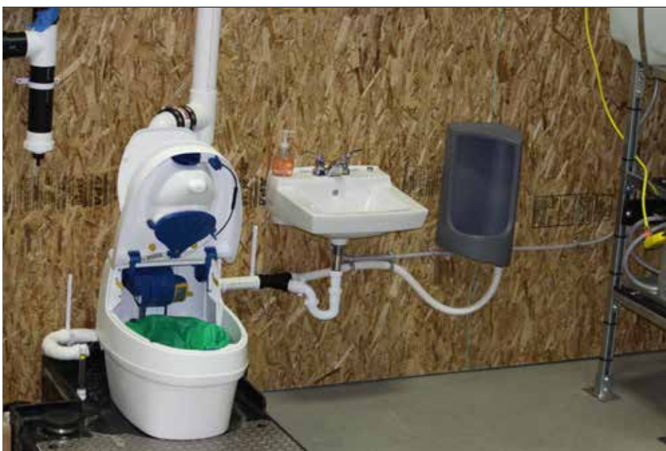
A test set-up of the stand-alone sanitation system.
